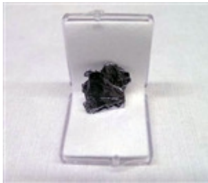
Single Crystal Molybdenum Disulfide (MoS 2 ) - Medium 15x10mm
